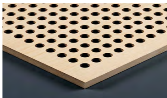
Typ: 10-16 ( \phi = 10 mm, Achsabstand = 16 mm)
