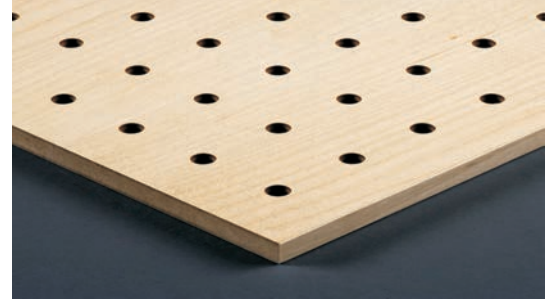
Typ: 8-32 ( \phi = 8 mm, Achsabstand = 32 mm)
