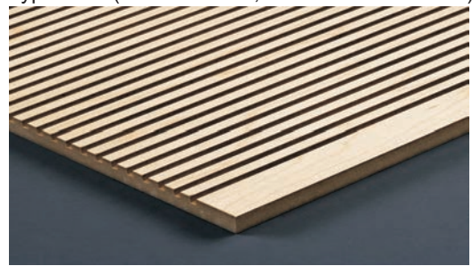
Typ: S 3-8 (Breite = 3 mm, Achsabstand = 8 mm)
